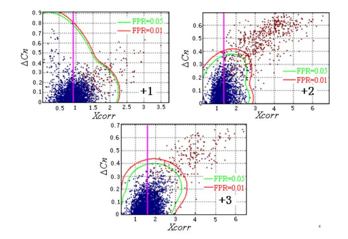
Inferred filter boundaries for different charge state observations in the control dataset. The red and green curves are the filter boundaries for FPR = 0.01 and for FPR = 0.05, respectively.
