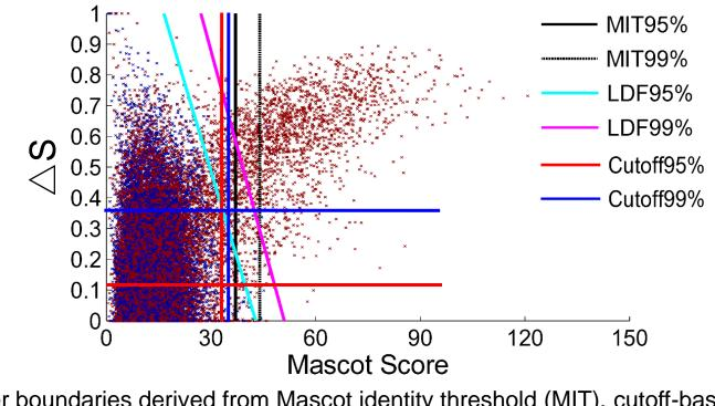
Filter boundaries derived from Mascot identity threshold (MIT), cutoff-based method, and LDF model for LTQ-FT control data set
